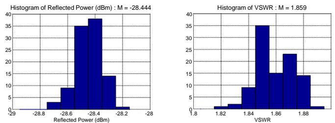
Fig. 4. Distribution of reflected power in 100 measurements for initial configuration of matching network  $C_1 = 4.50\text{pF}$ ,  $C_2 = 3.90\text{pF}$  at 1.8 GHz.
