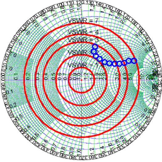
Fig. 2. Smith chart showing a) Constant VSWR circles (red) and b) Selected points (blue) representing variations of reflected coefficient of a plenary inverted-F antenna (PIFA) prototype held in hand at 1.8 GHz.
