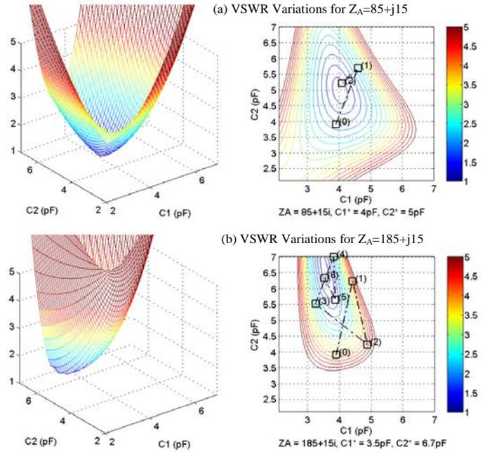
Fig. 7. Sample runs of iterative tuning based on VSWR variations. The optimal configuration is determined in (a) 2 and (b) 6 adjustments.
