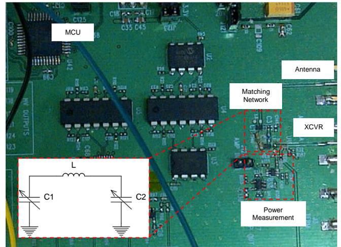
Fig. 3. System prototype comprising a matching network with two BST capacitors marked as  $C_1$  and  $C_2$  on the board, a microprocessor unit (MCU) as the decision control module, and a power measurement circuit.
