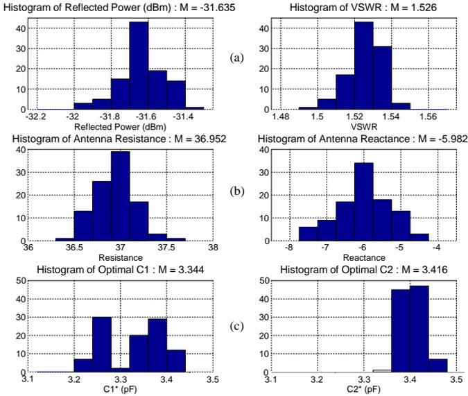
Fig. 5. Results of 100 sample run of matching method based on calculation of antenna impedance: (a) Distribution of power for perturbed configuration of matching network  $C_1 = 4.20\text{pF}$ ,  $C_2 = 3.50\text{pF}$  (b) Distribution of antenna impedance (c) Distribution of optimal configuration of matching network.
