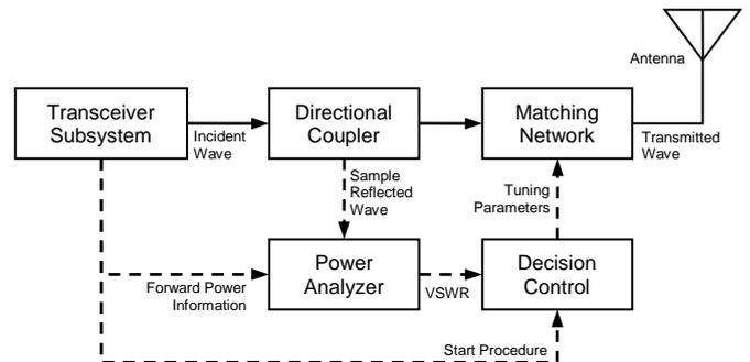
Fig. 1. Apparatus comprising the matching network, directional coupler, power analyzer and decision control module, with subsystem for gathering forward power information from the transceiver which may include power control data sent by the network, current drain, and so on.
