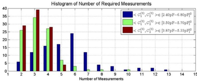
Fig. 6. Distribution of number of required measurements for unique identification of antenna impedance in 100 sample runs of the two-stage tuning algorithm (II.A) with random initial settings and perturbations.
